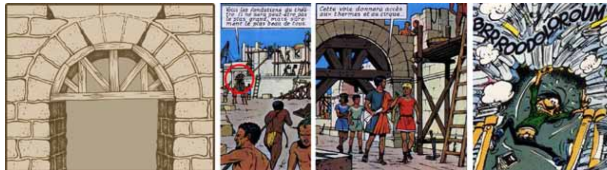
Left: Representation of a wood frame used to sustain the voussoirs until the insertion of the keystone. Center: Martin, J. (1970) Les Aventures d'Alix: Le Dieu Sauvage (Tournai: Casterman, 6, 5-7) Right: Franquin, A. (1979) Lagaffe: Mérite des baffes (Marcinelle: Editions Dupuis, 41, 6) [Image annotated by author]
